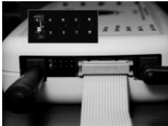
Figure 2-6: Jumper Settings for (5V) Target Power Connection via Power In and Power Out Jacks Of Cyclone
