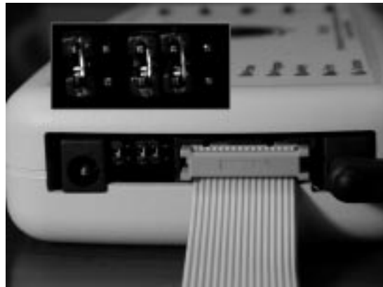
Figure 2-10: Jumper Settings for (5V) Target Power Connection via Cyclone Board Power and Power Out Jack of Cyclone
